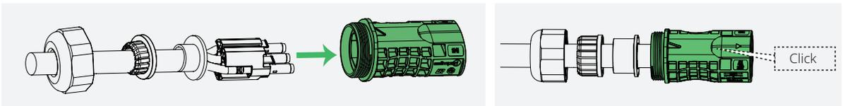
F) Slide the gasket, compression ring, and nut over the cable assembly. Tighten the nut to 2.5 ± 0.5 N·m.
