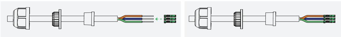
D) Insert the crimped cable into the connector body.
